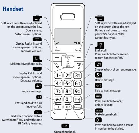
😑 The answer machine handset controls on buttons 24 44 54 and 61 will only work when a message is being played on the handset.
